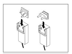
► Take the plug which is approved for the country in which the device will be used and insert it into the mains adapter.
