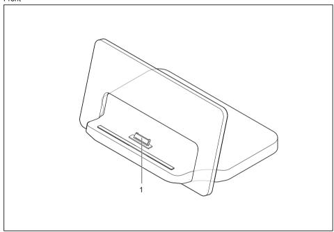
1 = Connector on the Cradle for the docking port of the Tablet PC
