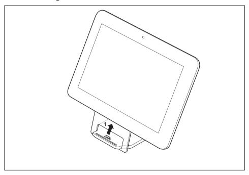
▶ Lift the Tablet PC from the Cradle (1), while supporting the underneath of the Cradle.
