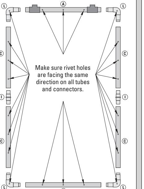
Step 1: Attach (C) tubes with (I) connectors as shown. Attach tubes (A) and (B) with the (L) connectors.
