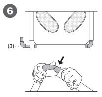
Step 6: Insert 1 (3) corner connector to the open end of the (C) tube. Rotate, or bend out slightly, the (3) connector that was just inserted. Line it up with the open end in the (B) side tube and press firmly until the pieces connect. [Note: This is a very tight fit. Please bend carefully.]
