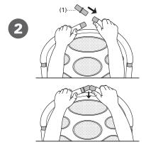
Step 2: Rotate, or bend out slightly, the 2 (A) tubes that were just inserted and place the (1) center connector into one of the open ends. Rotate the 2 (A) tubes back together making sure the center connector fits tightly inside the tubes. [Note: This is a very tight fit. Please bend carefully.]
