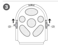
Step 3: Insert 2 (2) side connectors into the openings on the side pockets connecting them to the (A) tubes.
