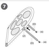
Step 7: Insert 2 (D) tubes onto the open stems of the 2 (2) side connectors already on the game board. Insert 2 (4) feet into the open ends of the (D) tubes.
