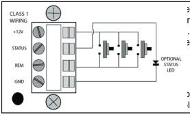
connect the REM to REM, +12V to +12V, GND to GND terminals of all units together. Be sure
