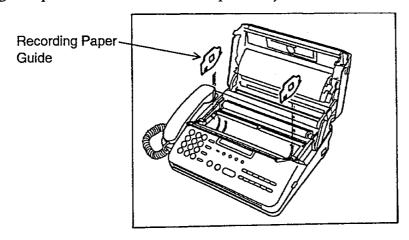
5. Load a Recording Paper, taking account of its feeding direction.
