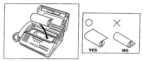
6. Feed the loaded Recording Paper under the Cutter Guide until paper head appears at paper exit.
