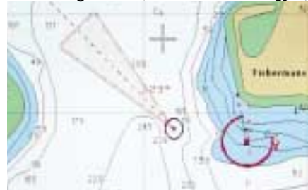
Continuously scans the chart data in front of the boat to detect dangerous objects (land, rocks,...).
