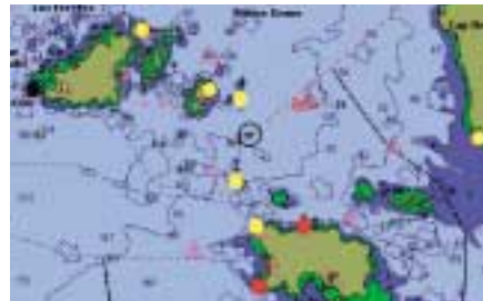
Flashing buoys and light houses are displayed with only visible sector colors according to boat's position.
