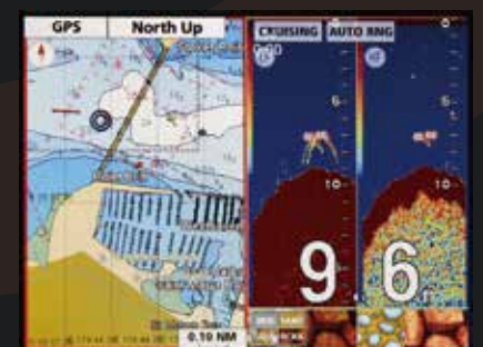
Plotter + Fish Finder* (with ACCU-FISH and Bottom Discrimination function ON) *GP-1670F only
