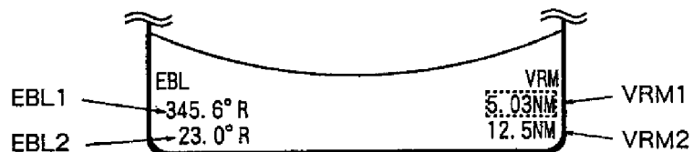
Figure 1-8 Display bottom, showing location of EBL and VRM readouts
