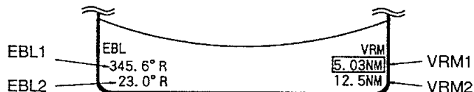
Figure 1-8 Display bottom, showing location of EBL and VRM readouts
