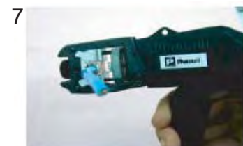
7 Using special crimping tool MPT5-8 (PANDUIT CORP.), crimp the modular plug. Finally check the plug visually.
