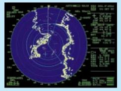
Electronic plotting of 10 targets according to the new IMO and IEC standards. Automatically redraw vectors between manual plots, drops off vectors if not plotted more than 10 min as required by IMO/IEC.
