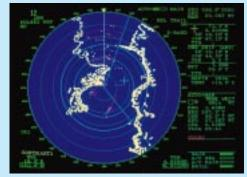
The Auto Plotter ARP-17 automatically tracks up to 20 targets acquired manually or automatically, presents target data, and triggers a collision alarm for the target on a collision course.
