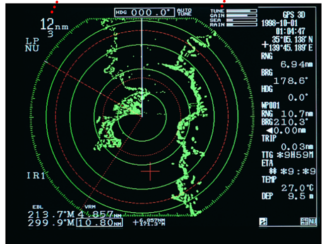
Range scale indicator Level Indicator Bars
