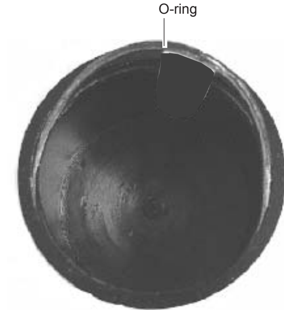
Battery cap, inside view
