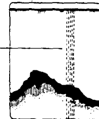
Interference from other electric devices
