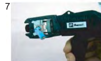
Using special crimping tool MPT5-8 (PANDUIT CORP.), crimp the modular plug. Finally check the plug visually.
