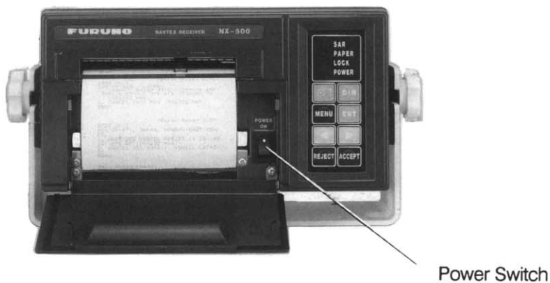
Fig. 2-3 NX-500, Panel opened to show Power Switch
