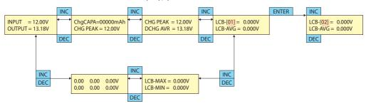
If the Battery TYPE button is pressed for over 3 seconds, the Data view will be displayed as above. Data displays can be scrolled left and right by using the INC & DEC buttons. If the Battery TYPE button is pressed again, the data view screen will disappear.
