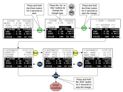
After selecting charge for a NiCd or NiMH pack, you are given the option to select four different charge types. These are:-
