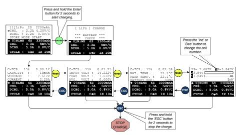
With the line selection arrow on the 'CHG.' line, check the correct charge current and cell voltage is selected, then press and hold the 'Enter' button for 2 seconds to start the charge.
