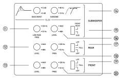
Bass Boost control allows precise shaping of the audio signal for your subwoofer(s). The Subsonic filter is essentially a high-pass crossover which blocks the frequency signal from 10Hz - 80Hz. This signal often contains no music & its removal will improve subwoofer control. The Bass Boost is a variable control to increase the level at 45Hz from 0 - +12dB of gain. Adjust these controls with extreme care.
