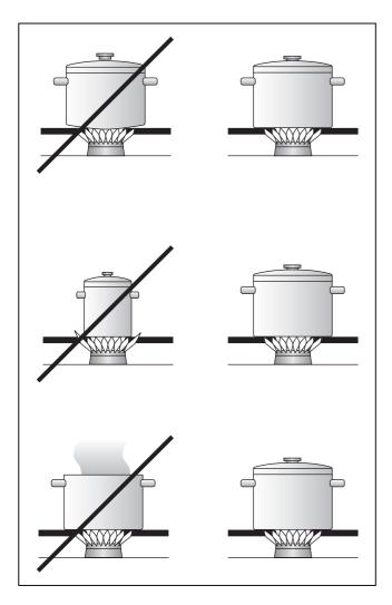
Pots with a diameter of less than **90 mm** or more than **280 mm / 320 mm for the large (WOK) burner** should not be used. When using large pots, pay attention to keeping to a minimum distance of **50 mm** between the cooking vessel and combustible surroundings.
