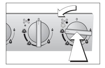
Only light a burner if all burner parts are dry, and assembled correctly. Otherwise, malfunctions may occur or the appliance may switch off.
