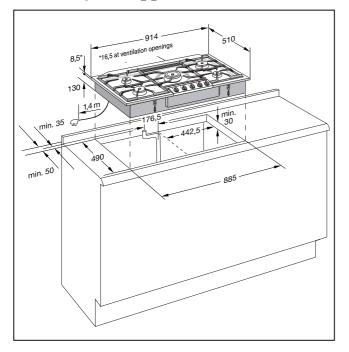
**Note:** the appliance can be installed in a base cabinet with a minimum width of 900 mm. The recess in the countertop will be slightly wider than the inner width of the base cabinet. Do not install the appliance above a drawer.
