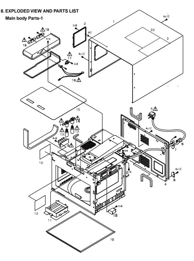
NOTE: All component have special characteristics for safety and must be replaced using parts listed in this manual. All service on M/W ovens should be performed by a qualified technician using approved testing equipment. Customers should not attempt replace component marked with a symbol.
