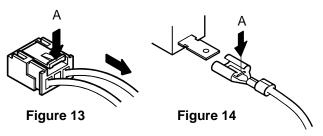
Pull connector case (Never pull the wire)
