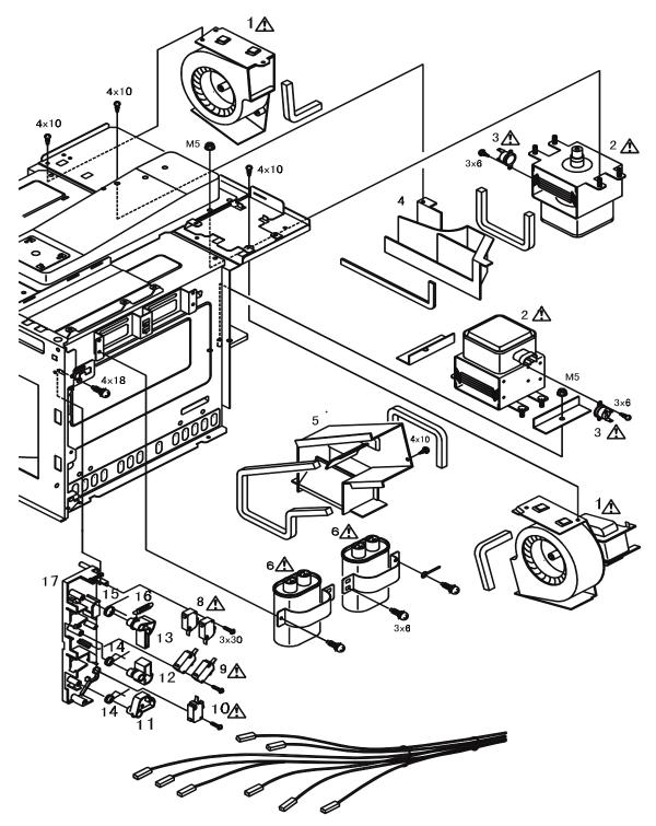
NOTE: All component have special characteristics for safety and must be replaced usnig parts listed in this manual.
