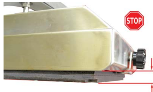
Incorrect: Grate not in place, front side too low compared to rear side.
