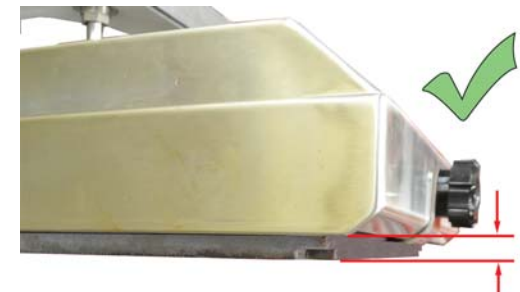
Correct: Grate in place, with consistent gap.
