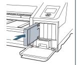
Note: If you can't insert the cartridge smoothly, you may have the wrong cartridge or are trying to insert it into the wrong slot. Check the package and part number. If the light remains on after installing the cartridge, try removing and then reinserting it.
