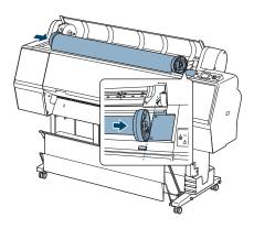
7 Slide the roll paper holder to align the ▲ arrow with the roll paper adapter.
