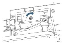
**10** Insert the cutter cover, then press it in until it snaps into place.
