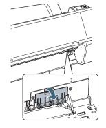
**6** Loosen the screw using a Phillips-head screwdriver.
