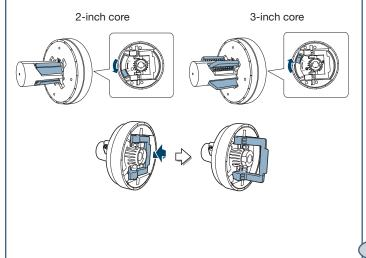
**5** Push the adapters into the paper core at both ends of the roll. Then press down on the tension levers to secure the adapters on the roll.
