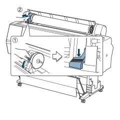
**5** Roll the paper forward so it rests on top of the printer.
