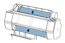
If the paper doesn't come out, lower the suction by pressing the  $\mathbf{\nabla}$  button. Return the suction to normal after the paper is loaded.
