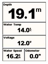
All sonar transducers display depth. Temperature-capable transducers display the Water Temp field. Speed-capable transducers or separate speed wheels display the Water Speed and Odometer fields.
