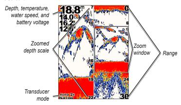
Press **MENU** to change the range, gain, beam, zoom, depth line, and sonar settings, as described starting on page 5.
