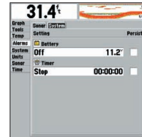
Main Menu - Alarms/System Tab
