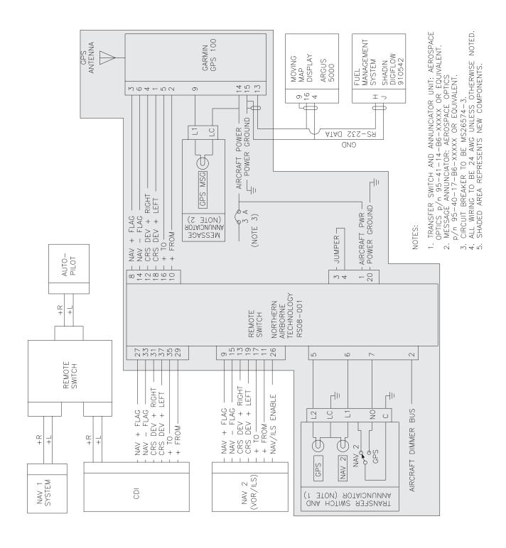
FIG A-4 WIRING DIAGRAM
