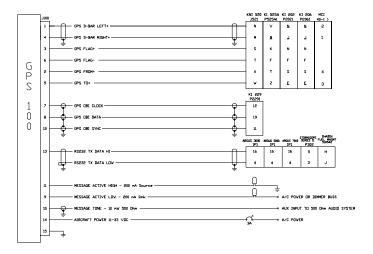
FIGURE 1-2 INTERCONNECT SCHEMATIC
