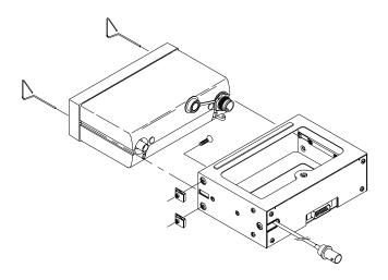
FIGURE 3-4 AVIATION RACK INSTALLATION
