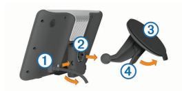
2 Press the mount ② onto the suction cup ③ until it snaps into place.
