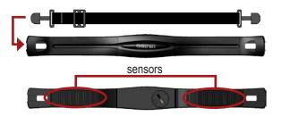
**2** Wet both sensors on the back of the heart rate monitor to create a strong connection between your pulse and the transmitter.
