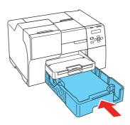
6 Slide out the output tray and flip up the extension.
