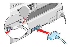
3. Connect the other end of the cable to your computer's main parallel connector (you can identify it by shape) and secure it as necessary.
