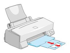
2. Load a stack of paper with the printable (whiter) side up and place it against the **right** edge guide. Then slide the left edge guide against the paper's left edge.
