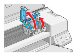
6. Place the ink cartridges into their holders with the blue labels facing up and toward the back of the printer. Then push down the clamps until they lock in place.
