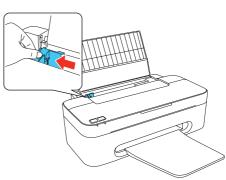
4 Load paper against the right edge guide and behind the tab, with the printable side face up.
