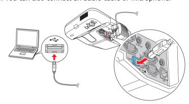
Follow the on-screen instructions to install the Epson USB Display software. If you see warning messages, click **OK** or **Continue**. (Software is installed only the first time you connect the computer.) Press the **USB** button on the remote control if necessary.
