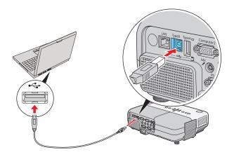
Follow the on-screen instructions to install the Epson USB Display software (with Mac OS X, first double-click the **USB Display Installer** icon that appears on your computer screen). Then press the **USB** button on the remote control. (You need to install the software only the first time you connect.)
