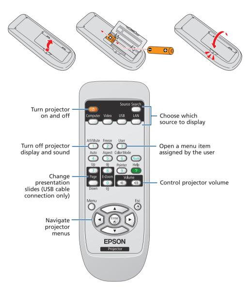
You can use the remote control to operate the projector. With the USB cable, you can use the remote as a wireless mouse. For more information on using the remote control, see the *User's Guide* on your projector CD.
