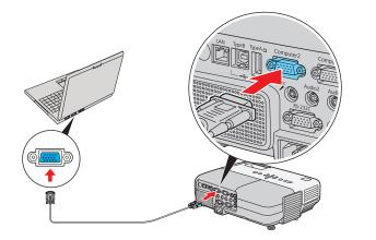
Connect one end to the projector's **Computer1** or **Computer2** port, and the other end to your computer's O monitor port. If you are using a notebook, switch it to external display. You can also connect an audio cable to the **Audio1** or **Audio2** port.
