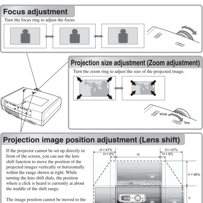
The image position cannot be moved to the maximum vertical values and maximum horizontal values at the same time. Ex) The image cannot be shifted
