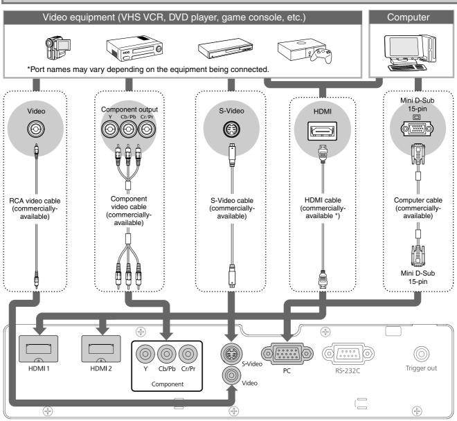
\* Use a HDMI cable that conforms to the HDMI specifications.
