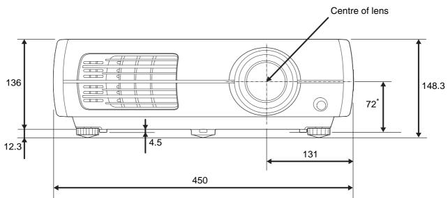
\* Distance from centre of lens to suspension bracket fixing point
