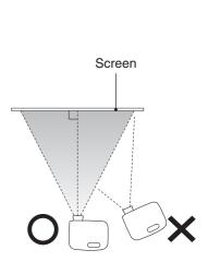
If the projector is placed at an angle to the screen, then the projected image will be distorted.
