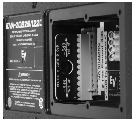
Figure 11b: EVA input panel, with the switch card inserted to shade the lower HF element 3 dB
