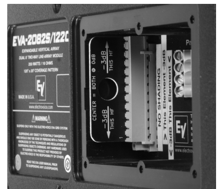
Figure 11c: EVA input panel, with the switch card inserted to shade the upper HF element 3 dB
