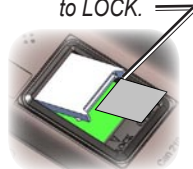
Detail of microSD card tray in Battery Compartment
