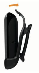
**3** To remove, pull up on the upper clip while pressing on the back of the device to release the top, and slide it out of the lower clips.
