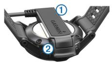
4 Align the hinged side of the charger ② with the contacts on the back of the device.
