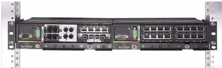
Fig 3.3.2b- Two Magnum 6K16s deployed over a K16-2Tray side-by-side to provide larger port density of 32 ports.
