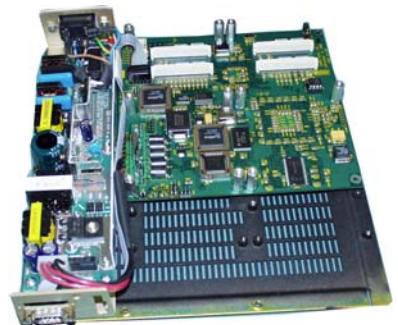
Figure 3.6.1b: Magnum 6K16-Series, Top view without chassis cover
