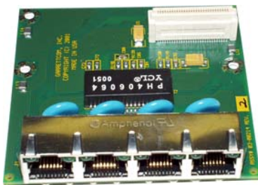
Fig 3.6.2b Granddaughter Board placed in slot A & secured with three 5/16 stand-off's
