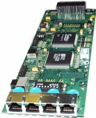
Fig. 3.6.2c Daughter Board, top view of version for 4 copper 10/100 ports
