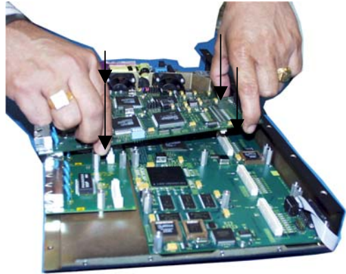
Figure 3.5.3b: Removing a 6KPM Card
