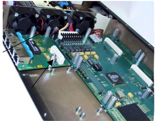
Fig 3.5.2b Granddaughter Board placed in slot A and secured with three 5/16 stand-off's
