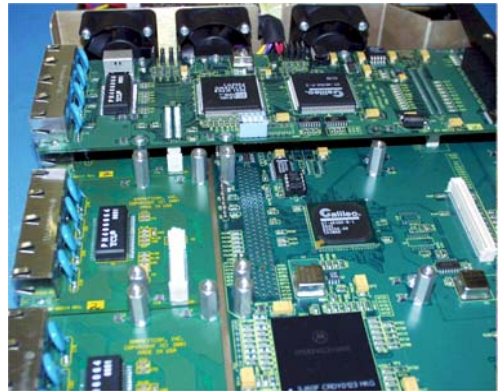
Fig. 3.5.2g Top View : 6KPM Module installed inside a 6K25
