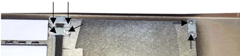
Figure 3.5.1c: Top View – 6KPM retaining screws hold Face Plate
