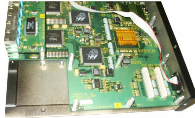
Figure 3.5.1c: Magnum 6K32's modular slot side (front-right side), without chassis cover
