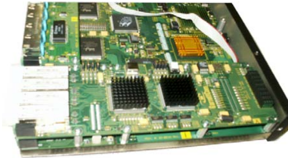
Fig. 3.5.2g Top View : 6KPM Module installed inside a 6K32T &
