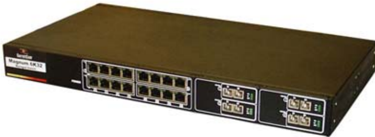
Figure 2.2.1b: 6K32T front view, configured for 16 RJ-45 ports + 2 Modular slot with Dual Giga module.
