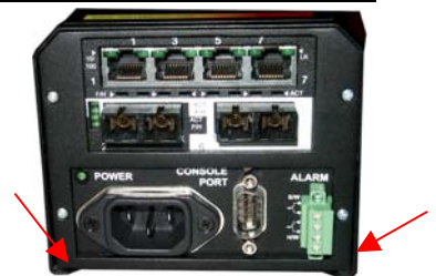
Figure 3.6.1c: Top View – 6KPM retaining screws hold Face Plate
