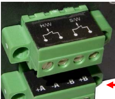
Figure C5.0: DC Dual-Source, wiring connections with Dual-Source option.
