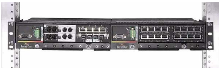
Fig 3.3.2b- Two Magnum 6K16s deployed over a K16-2Tray side-by-side to provide larger port density of 32 ports.
