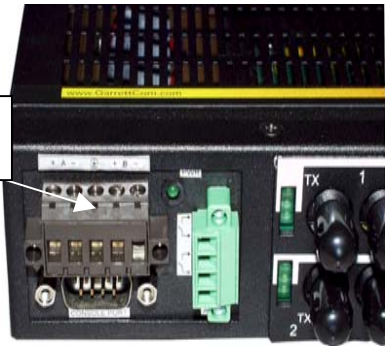
Figure C5.0: -48VDC Dual-Source, wiring connections to the External Terminal Block on a Magnum -48VDC with Dual-Source option
