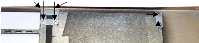
Figure 3.6.1c: Top View – 6KPM retaining screws hold Face Plate
