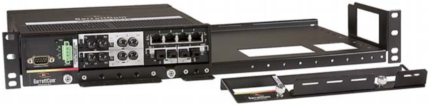
Fig 3.3.2a- One Magnum 6K16 deployed over a K16-2Tray
