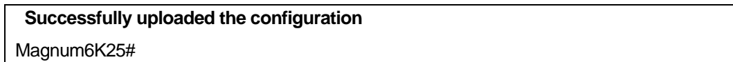
FIGURE 165 – Message which shows the completion of the file transfer (from 'saveconf' command)
