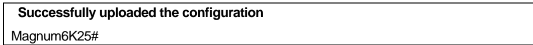
FIGURE 151 – Message which shows the completion of the file transfer (from 'saveconf' command)
